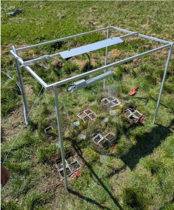
Figure 3 - Experimental group of swards in the extended photoperiod treatment using twilight-activated lamps
